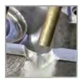
Cold Spray uses Kinetic Transfer instead of Thermal Transfer. Temperatures of material being applied stay at 250 degrees or less. The process yields a repair where the added material is as good if not better than the base part being repaired.
