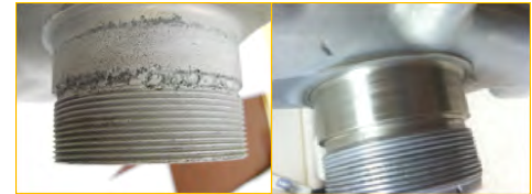
After Cold Spray, parts can be returned to their original state
