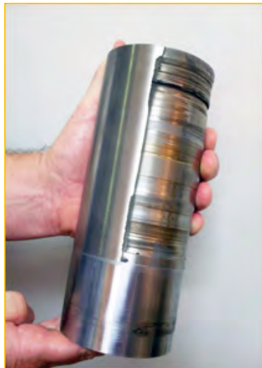
Significant amounts of materials can be reapplied to heavily damaged parts
